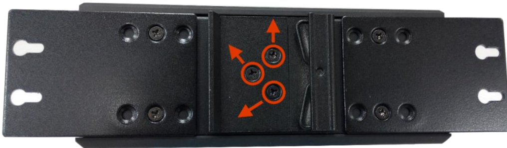
Figure 3.4: Remove DIN-Rail Bracket from the Switch
