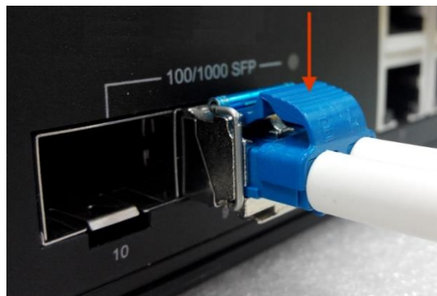
Figure 2.4: Remove LC Connector
