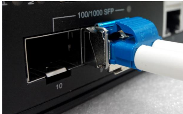
Figure 2.9: LC Connector to the Transceiver
