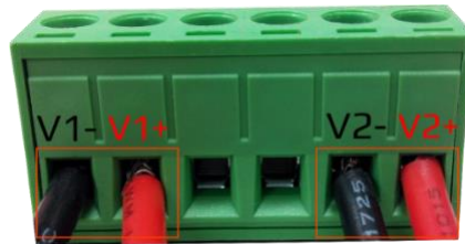
Figure 2.9: Power Terminal Block
