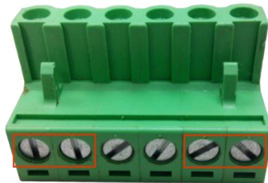
Figure 2.10: Power Terminal Block
