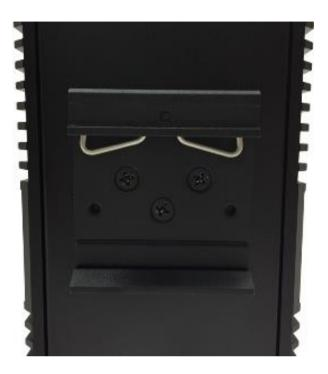
b. Insert the top of the DIN-Rail bracket to the DIN-Rail track.
