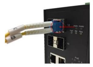
2. Open the SFP module and remove it.
