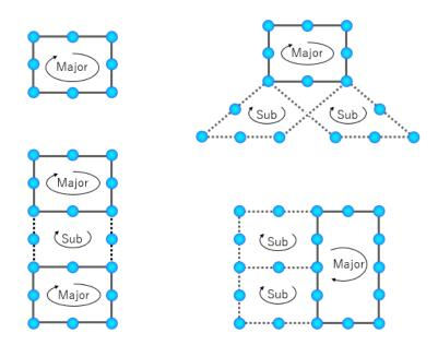
Using major ring and sub ring can design multiple ring or ladder topology. With these topologies, ERPS can append to variance application with different level of ring network. For example, core ring and branch ring architecture has application in campus and the area with central control node. Ladder topology has lots of case for tunnel and train application. The benefit of small ring is less effect nodes if ring caused of recovery.
