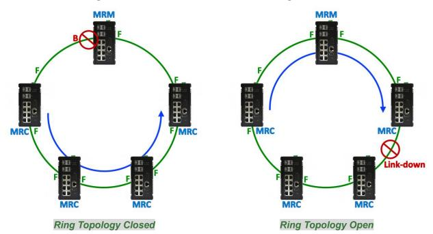
If the **MRC** detects a link down at one of the ring ports, it can notify this event to the **MRM** initiatively. In **Advanced Mode**, the MRM can activate the blocked ring port to speed-up recovery rather than wait till sufficient loss of test packets.
