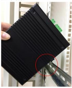
c. Pull down the DIN-Rail bracket to the DIN-Rail track and check if it is mounted tightly on the DIN-Rail track.
