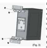
In case you purchased the optional mounting kit (mounting plates), there are mounting plates and screws that come inside the package; proceed to place the screws on the back of the device as shown in Fig. 3.
